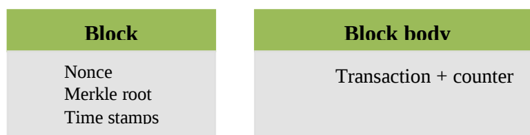
Figure 3: Block Data structure
